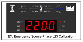
Step 4: Use a good quality voltmeter as a reference to calibrate the ATS-465 voltage reading to the desired phase.
