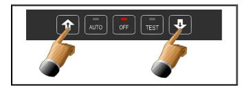
Step 6: Press the "OFF" button to move to the next phase or until the word "End" appears on the screen. To exit hold the "OFF" button at any time for 4 sec.
